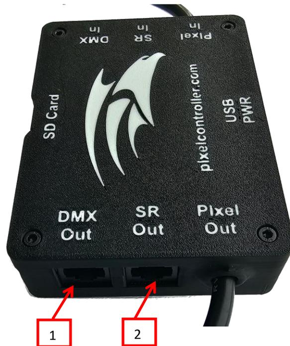
1. Smart Remote Output port. This port is used to output Smart Remote data to Smart Remote to see if they are functioning correctly. If using HinksPix receivers, you will need an adapter cable, refer to the [References](#) section.
