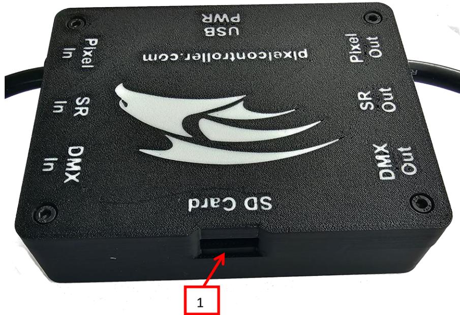
1. Micro SD Card slot. This is used for firmware updates when needed and for logging if selected.
