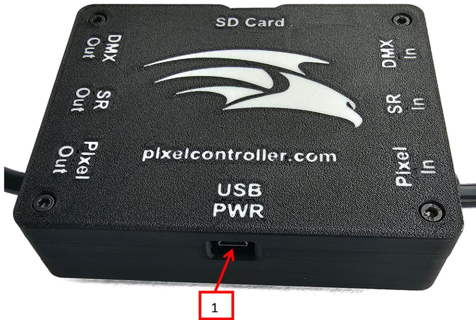
1. USB Power jack. The F-Test requires some sort of power. If connected to an energized pixel string, this will supply the power needed. If you do not have an energized pixel string connected to the F-Test, then you can supply power through the USB port.
