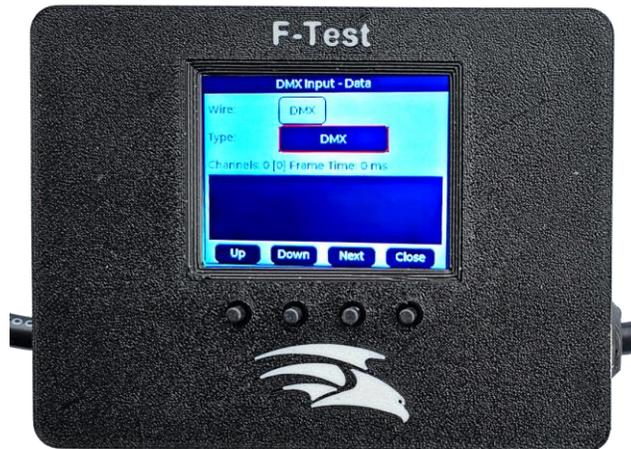
Pressing the Up and Down buttons will navigate through the available options in the highlighted menu item. The Next button will move the highlighted selection to the next item in the Menu. If you are on the Type option, the Next Button will toggle to the next display screen. The close button will take you back to the Main Menu.
