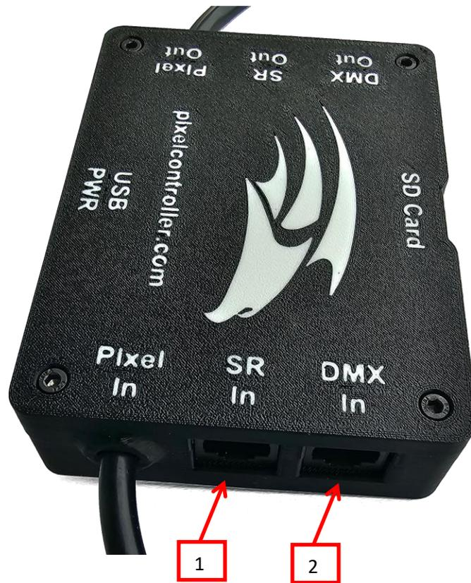
1. Smart Remote Input port. This port is used to monitor the Smart Remote data that a controller is sending to the remote receivers. If using HinksPix controllers, you will need an adapter cable, refer to the [References](#) section.
